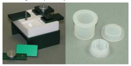
Polyethylene embedding forms 25 mm & "cradle" insert for the round specimen holder on the rotation microtome.
